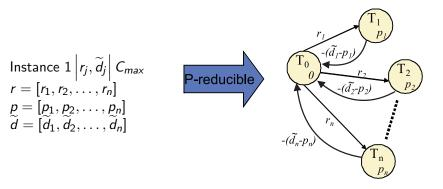
Reduction from PSm, 1 |temp|  $C_{max}$  to PS1 |temp|  $C_{max}$  is based on the projection of **each resource to the independent time window**. In other words, the schedule of tasks on  $P_j$  is projected into interval  $\langle (j-1) \cdot UB, j \cdot UB \rangle$
