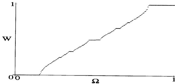
Figure 9.20: The Devil's staircase for K = 1 .
