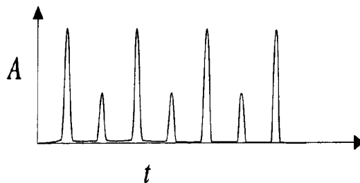
Figure 27.1: A signal showing a period-2 characteristic.
