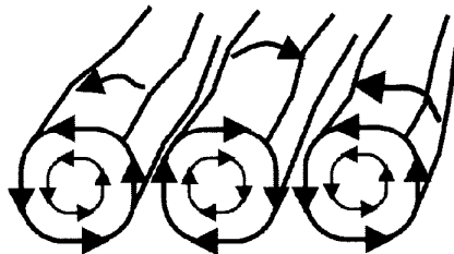
Figure 3.7: Cylindrical rolls in Rayleigh–Bénard convection.
