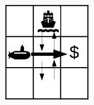
The reference plan is not eventually applicable (the ship either block or poses a direct threat to the AUV)
