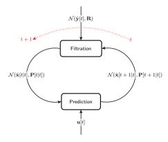
Simulates a single step based on the current control action  $\mathbf{u}[t]$  using the system model  $(\mathbf{A}, \mathbf{B}, \mathbf{C})$  and updates our estimated probability density function (described by the mean and covariance matrix):
