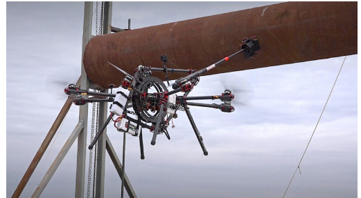
Figure 5: Fully-actuated multirotor UAV applying force to a pipe.
