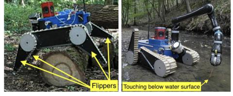
Construction: 2× main tracks, 4× subtracks (flippers), differential break great stability and climbing capability
