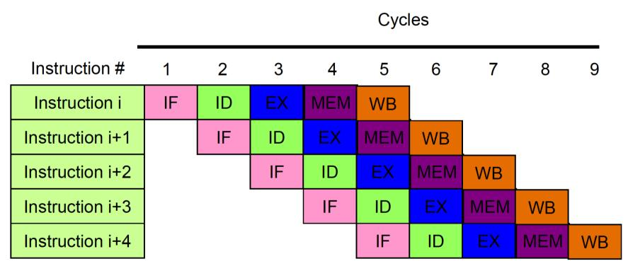
» each step is parallelized as well, e.g. Haswell does 4 instructions in single cycle (execution depends on type and independency of instructions)
