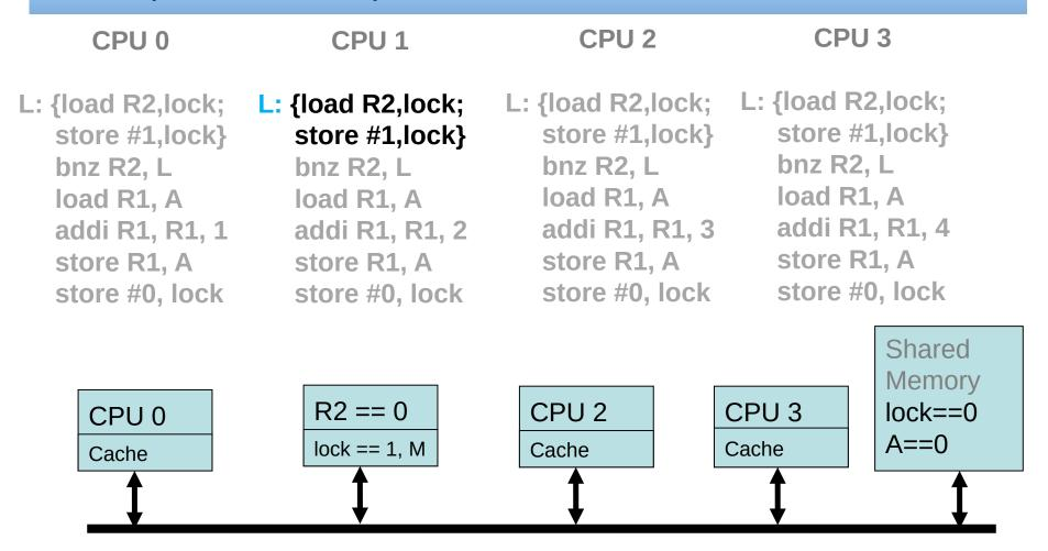
• CPU 1 obtains the bus. It reads the value of "lock" variable from memory to R2 and writes 1 to memory. The write happens only in its cache. The cache line reaches state M (modified).
