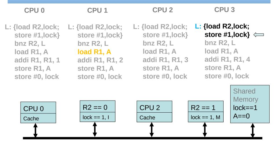
• CPU 3 keeps bus control (lock prefix). The next step of the atomic operation test-and-set is to write 1 to "lock" memory location. That is recognized by the snooping CPU 1, which changes its state to I (invalid). CPU 3 reaches state M. CPU3 releases the bus.
