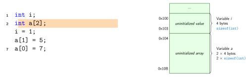
In the example, the variable allocation starts from the address  $0 \times 100$  for visualization and understandability. Automatic variables on the stack are usually allocated from the upper address to the lower ones.
