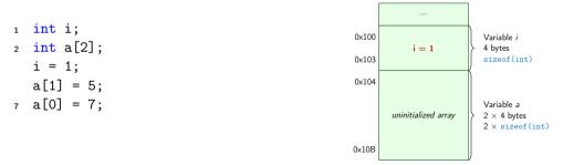
In the example, the variable allocation starts from the address  $0 \times 100$  for visualization and understandability. Automatic variables on the stack are usually allocated from the upper address to the lower ones.
