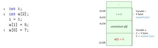
In the example, the variable allocation starts from the address  $0 \times 100$  for visualization and understandability. Automatic variables on the stack are usually allocated from the upper address to the lower ones.
