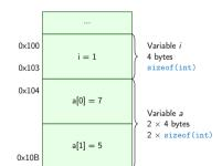
In the example, the variable allocation starts from the address  $0 \times 100$  for visualization and understandability. Automatic variables on the stack are usually allocated from the upper address to the lower ones.
