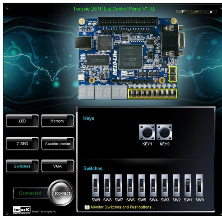
**Figure 2-5 Monitoring switches and buttons**
