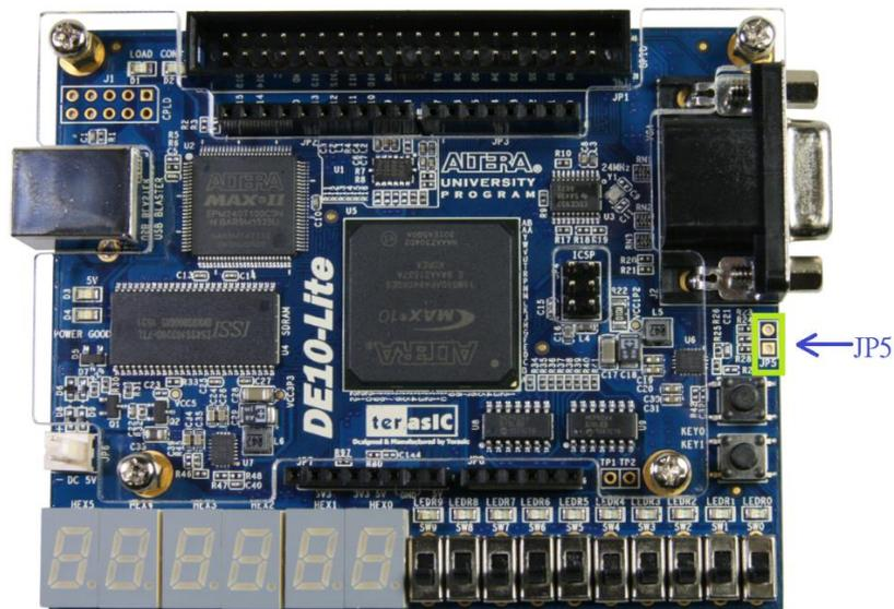
**Figure 6-1 JP5 position on the DE10-Lite board.**
