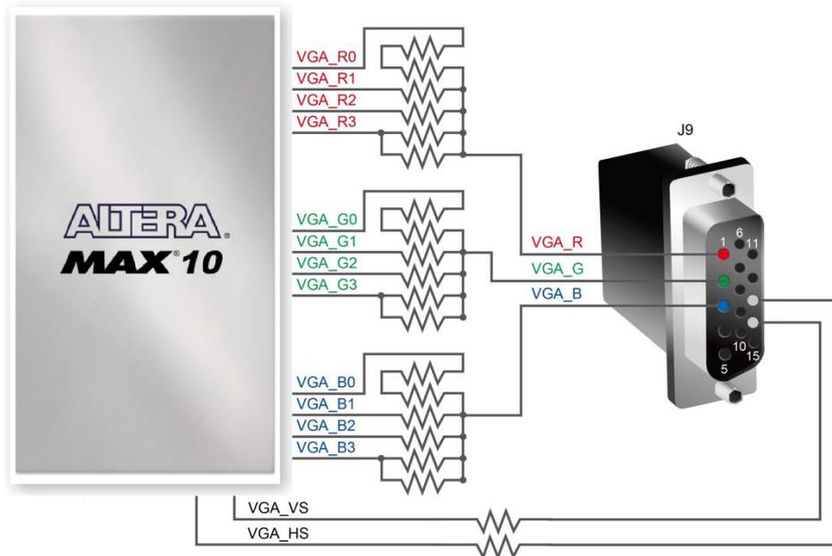
**Figure 3-21 Connections between the VGA and MAX 10 FPGA**
