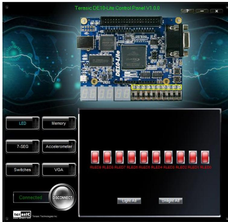
Figure 2-3 Controlling LEDs
