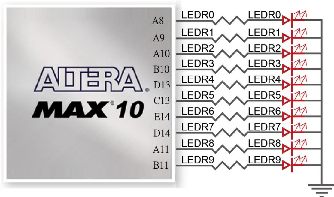
**Figure 3-16** Connections between the LEDs and MAX 10 FPGA
