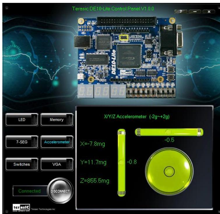
**Figure 2-7 Level by G-Sensor**
