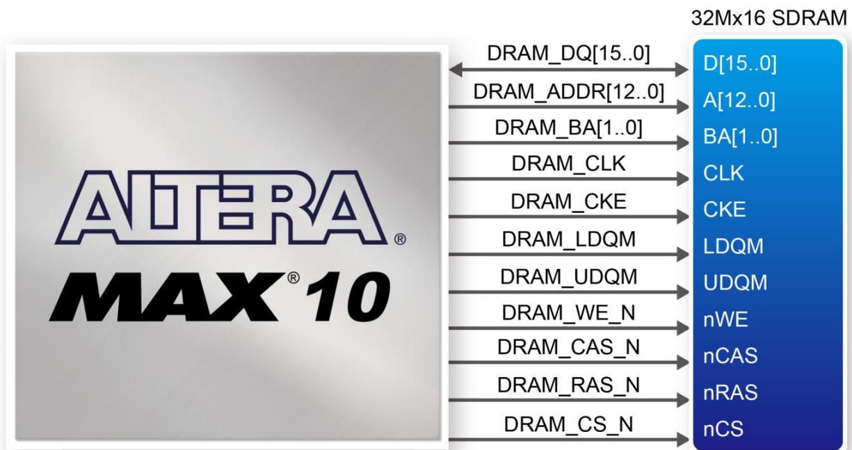
Figure 3-23 Connections between the SDRAM and MAX 10 FPGA
