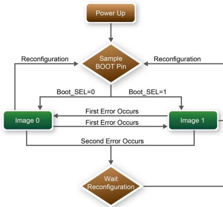
**Figure 6-3 Remote System Upgrade Flow for MAX 10 Devices**
