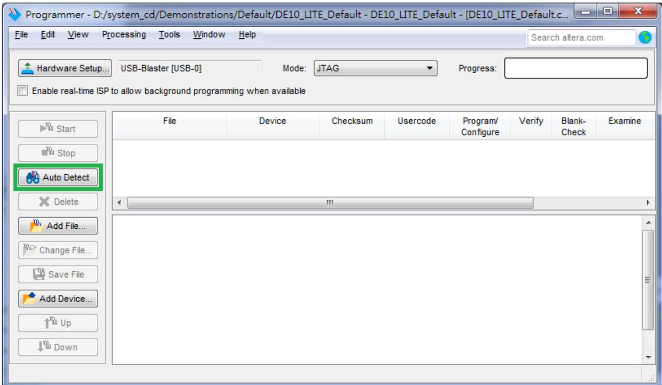
Figure 3-4 Detect FPGA device in JTAG mode
