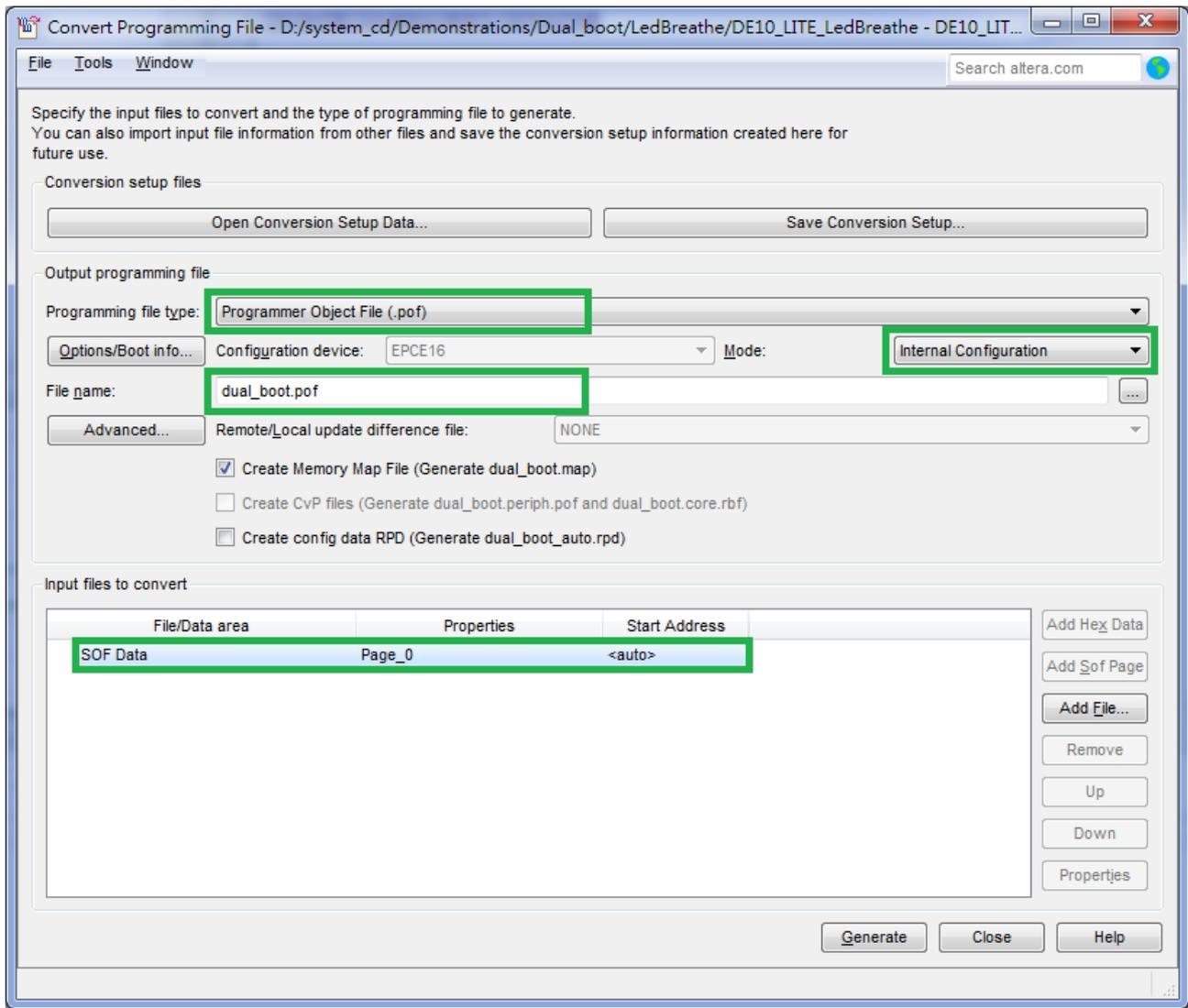
Figure 6-14 Dialog of Convert Programming Files and setting
