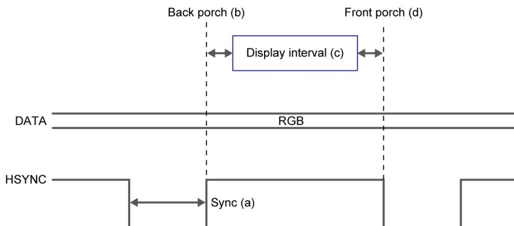
**Figure 3-22** VGA horizontal timing specification
