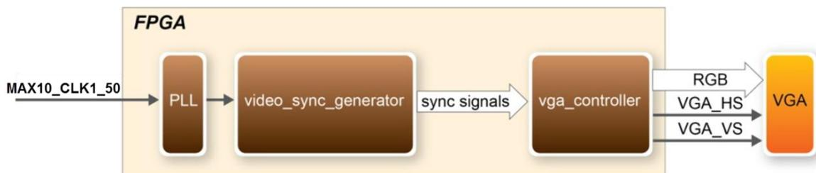
**Figure 5-5** Block diagram of the VGA Pattern demonstration
