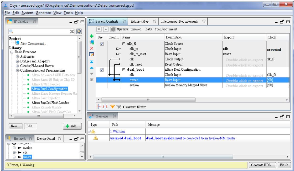
**Figure 6-7 Rename and connect dual boot IP OK**
