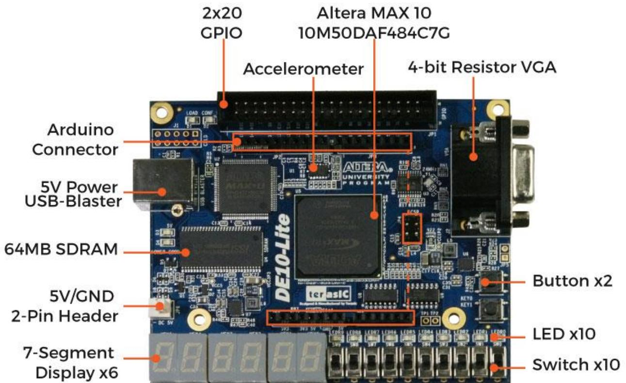
Figure 1-2 Development Board (top view)
