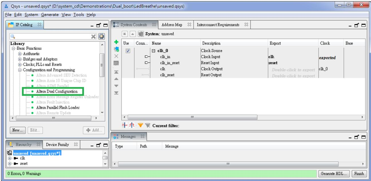
**Figure 6-5 Select Altera Dual Configuration IP and click.**
