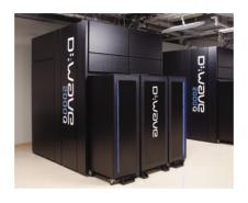
This is the D-Wave 2000Q system. It performs quantum annealing using superconducting qubits that live in the very end of a dilution refridgerator cooled at approximately -273.5 degrees Celcius.
