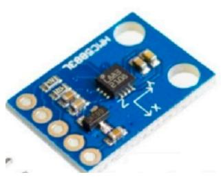
Magnetometer (angle to magnetic north)
