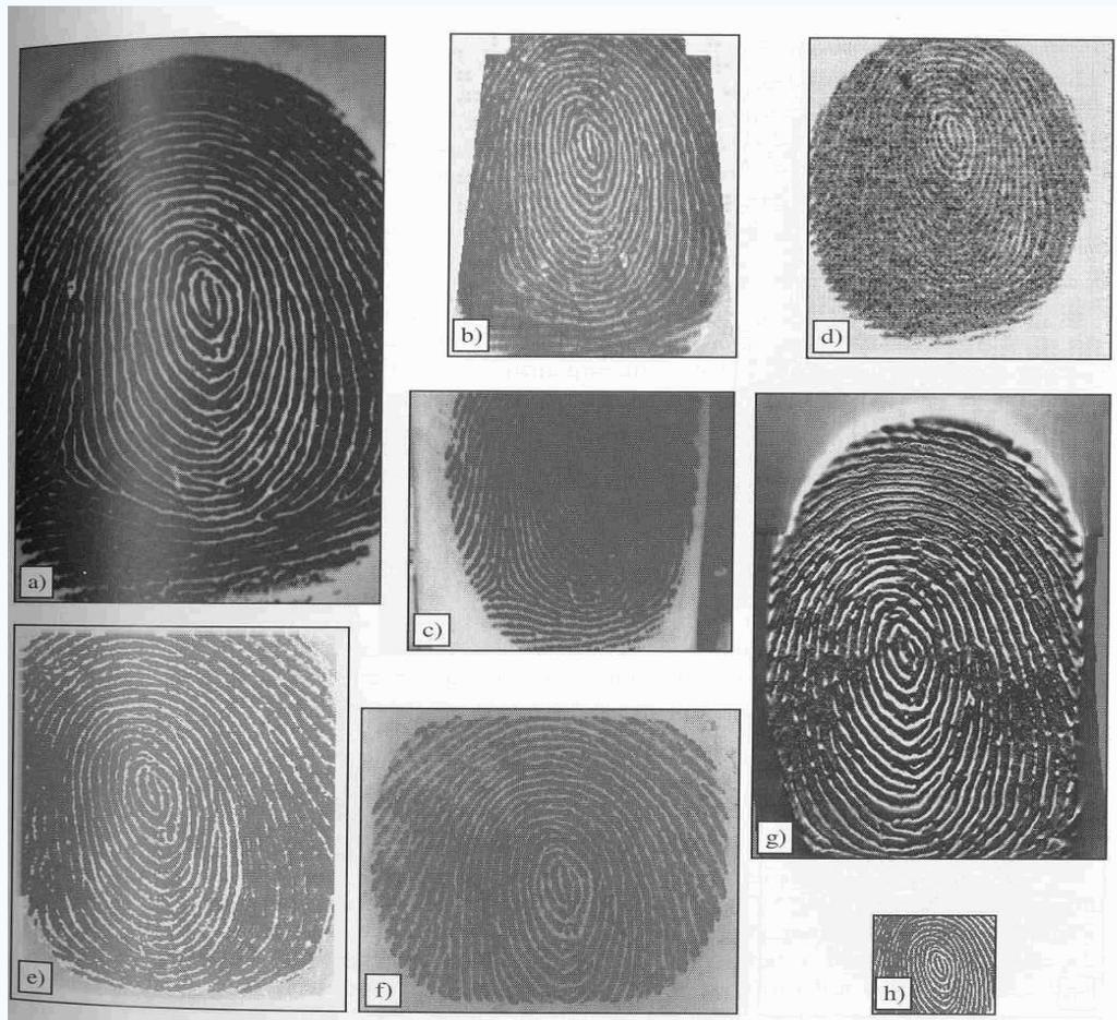
Figure 2.16. Fingerprint images of the same wet finger as acquired by different commercial scanners. Images are reported with right proportions: a) Biometrika FX2000, b) Digital Persona UareU2000, c) Identix DFR200, d) Ethentica TactilSense T-FPM, e) ST-Microelectronics TouchChip TCS1AD, f) Veridicom FPS110, g) Atmel FingerChip AT77C101B, h) Authentec AES4000.
