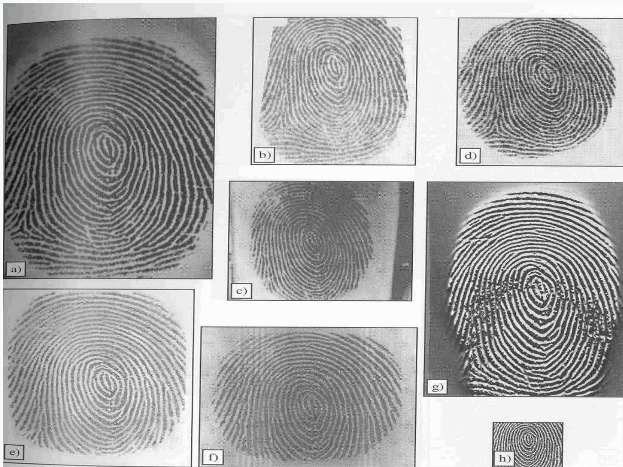
Figure 2.14. Fingerprint images of the same finger with ideal skin condition as acquired by different commercial scanners. Images are reported with right proportions: a) Biometrika FX2000, b) Digital Persona UareU2000, c) Identix DFR200, d) Ethenica TactilSense T-FPM, e) ST-Microelectronics TouchChip TCS1AD, f) Veridicom FPS110, g) Atmel FingerChip AT77C101B, h) Authentec AES4000.
