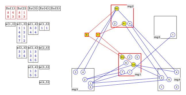
Fig. 3: The camera cluster and the point cloud initialised. The cameras belonging to the cluster are marked red, the scene-to-image correspondences that are confirmed are red as well.
