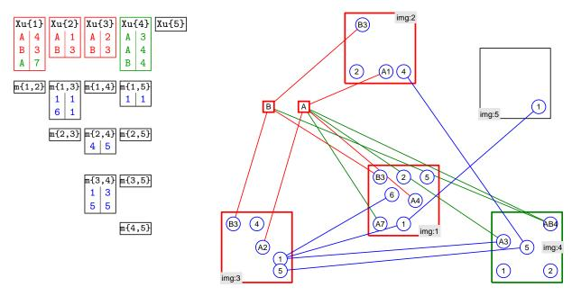
Fig. 10: Correspondences propagated from the attached camera (red for confirmed, green for tentative).
