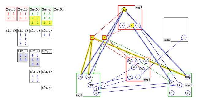
Fig. 5: Correspondence propagation from the first camera. The same colours as in the previous figure.
