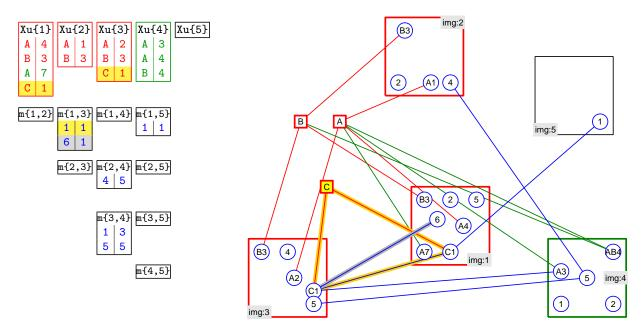
Fig. 11: Reconstructing new points from inlier image-to-image correspondences (emphasised yellow) between the attached camera and the cluster. The new (confirmed) scene-to-image correspondences are emphasised yellow.
