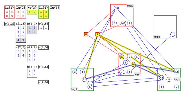
Fig. 4: Correspondence propagation from the first camera. The used and later removed correspondences are emphasised in gray, while the new correspondences are emphasised in yellow.
