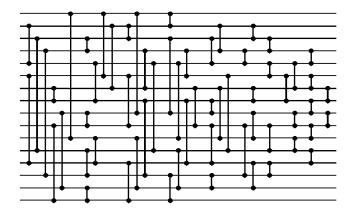
Each vertical line represents a comparator that switches the input numbers if they are not in desired order.
