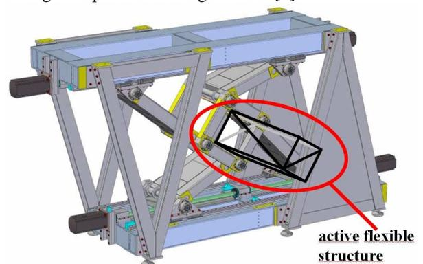
Fig. 1: Parallel redundant machine Sliding Star
