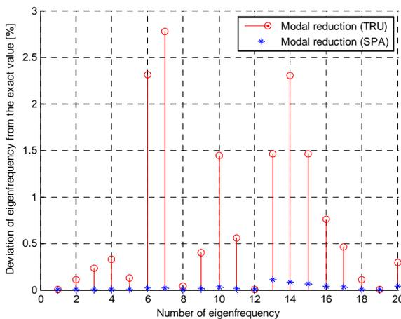
Fig. 4: Errors of first 20 eigenfrequencies for connected bodies modeled by two types of reductions SPA/TRU
