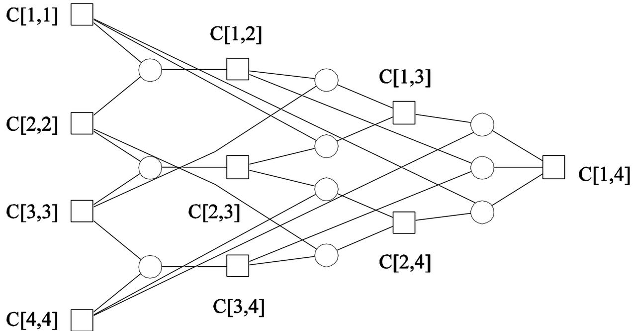
A nonserial polyadic DP formulation for finding an optimal matrix parenthesization for a **chain of four matrices**. A **square node** represents the **optimal cost** of multiplying a matrix chain. A **circle node** represents a **possible parenthesization**.
