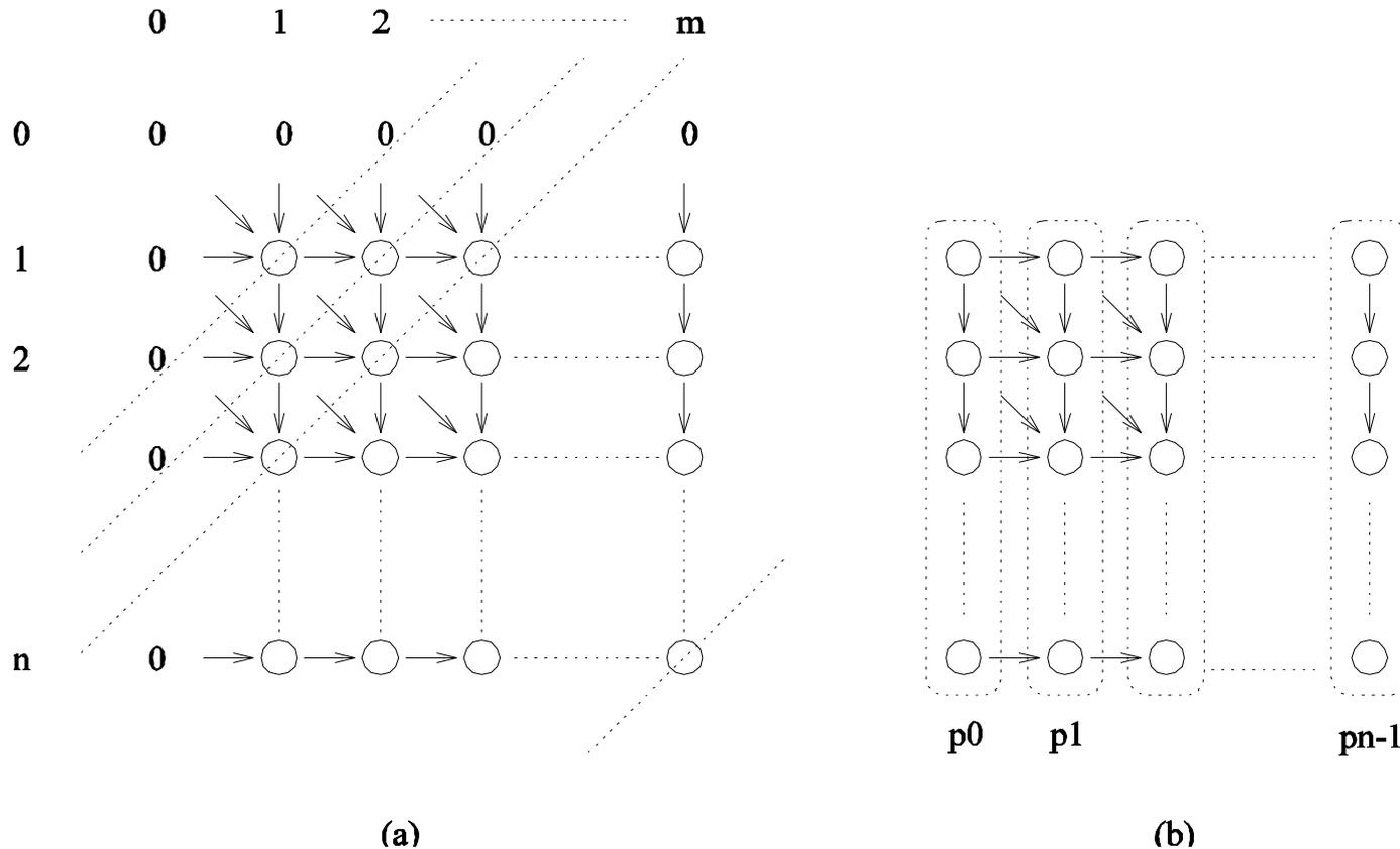
(a) Computing entries of table for the longest-common-subsequence problem. **Computation proceeds along the dotted diagonal lines.** (b) **Mapping elements** of the table to processing elements.
