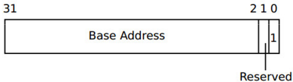
Base Address for PCI I/O Space
