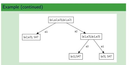
The algorithm ends up with two MUPSes  $\{\alpha_1, \alpha_2\}$  a  $\{\alpha_1, \alpha_3\}$ . "For free" we got diagnoses  $\{\alpha_1\}$  a  $\{\alpha_2, \alpha_3\}$ .
