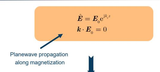
Fundamental modes are circularly polarized waves  $\frac{k_z^2}{k_0^2} = 1 - \frac{\omega_{\rm p}^2}{\omega \left(\omega \pm \omega_{\rm c}\right)}$   $\hat{E}_x = \mp {\rm j} \hat{E}_y$
