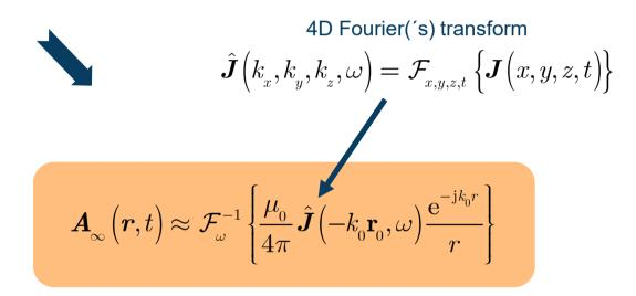
Radiation diagram is formed by Fourier(`s) transform of sources
