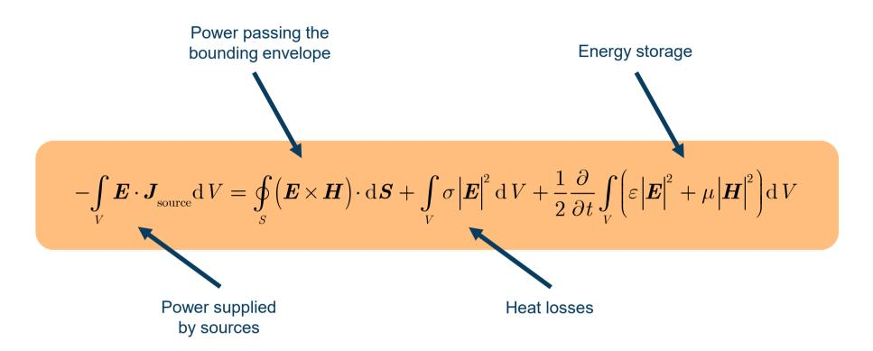
Energy balance in an electromagnetic system
