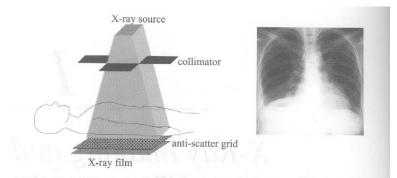
FIGURE 1.1. (Left) The basic setup for X-ray imaging. The collimator restricts the beam of X-rays so as to irradiate only the region of interest. The antiscatter grid increases tissue contrast by reducing the number of detected X-rays that have been scattered by tissue. (Right) A typical planar X-ray radiograph of the chest, in which the highly attenuating regions of bone appear white.
