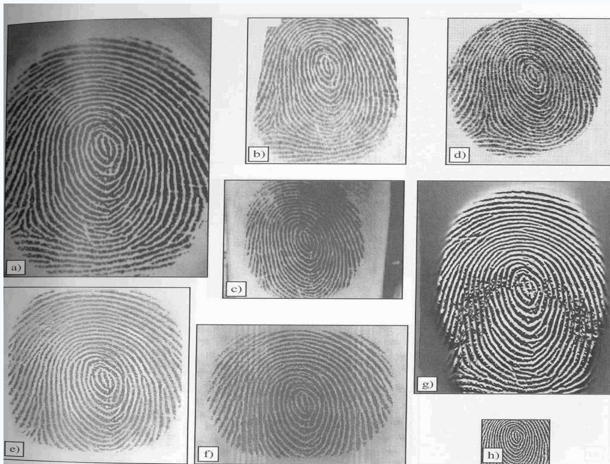
Figure 2.14. Fingerprint images of the same finger with ideal skin condition as acquired by different commercial scanners. Images are reported with right proportions: a) Biometrika FX2000, b) Digital Persona UareU2000, c) Identix DFR200, d) Ethenica TactilSense T-FPM, e) ST-Microelectronics TouchChip TCS1AD, f) Veridicom FPS110, g) Atmel FingerChip AT77C101B, h) Authentec AES4000.
