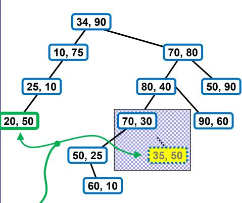
The query point [35, 50] is inside leaf cell defined by node [70, 30]. The closest point to query [35, 50] is the point [20, 50] which lies in a distant part of the tree.
