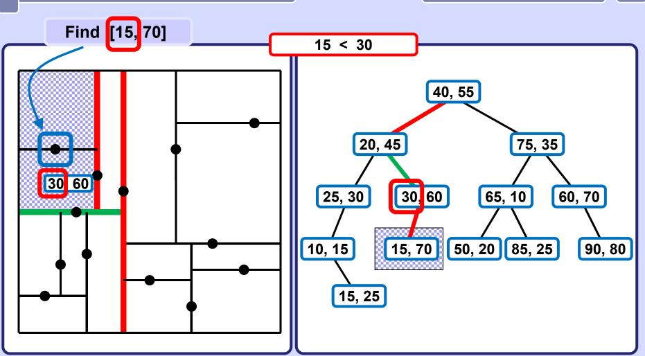
Q = [15, 70], N = [30, 60], Q != N, h(N) = 0. Compare **x-coordinate** of searched key Q to **x-coordinate** of the current node N and continue search accordingly in the left or in the right subtree of N.
