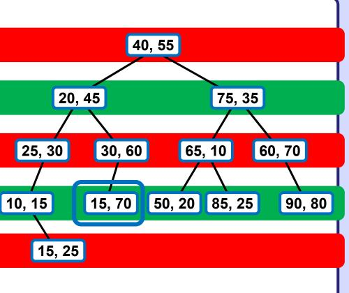
Operation Find works analogously as in other (1D) trees. Note how cutting dimension along which the tree is searched alternates regularly with the depth of the currently visited node.
