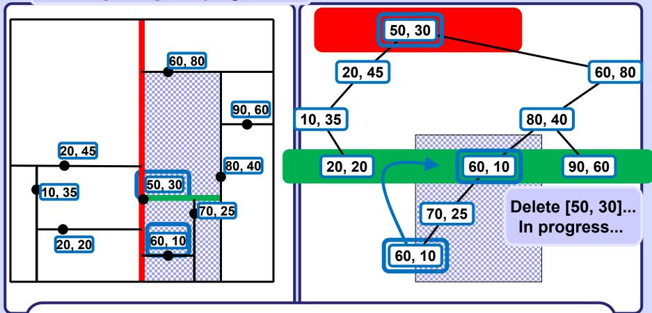
Deleting node [50, 30], its cutting dimension is y, it has no R subtree. Find node Z with minimum y-coordinate in LEFT subtree of [50, 30], Fill [50, 30] with keys of Z and move L subtree of [50, 30] to its R subtree. If Z is not a leaf continue by recursively deleting Z.
