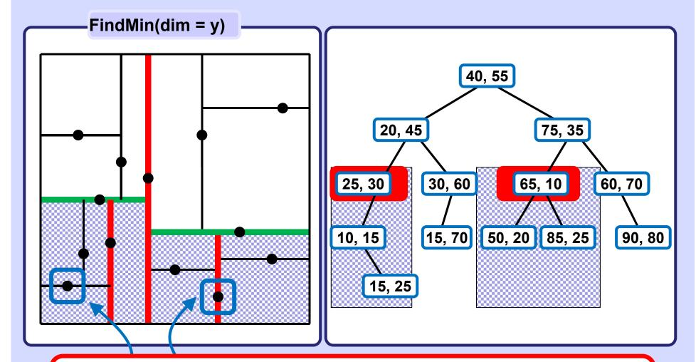
Node with minimal y-coordinate can be in L or R subtree of a node N corresponding to cutting dimension other than y, thus both subtrees of N (including N) must be searched.
