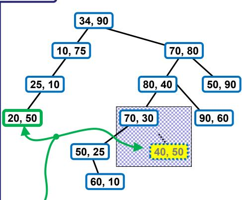
The query point Q = [40, 50] lies inside (empty) leaf cell right to the node [70, 30]. The closest point to query Q = [40, 50] is the point [20, 50] which, in fact, lies in a distant part of the tree.
