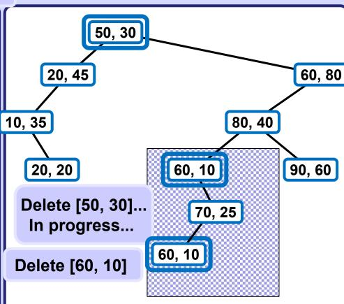
Deleting original node [60, 10], it it is a leaf, delete it and and stop. Note the change in the cell division left to [80, 40], the node with minimal y-coordinate becomes the splitting node for the corresponding area.
