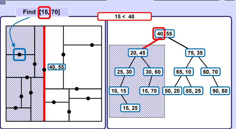
Q = [15, 70], N = [40, 55], Q != N, h(N) = 0. Compare **x-coordinate** of searched key Q to **x-coordinate** of the current node N and continue search accordingly in the left or in the right subtree of N.
