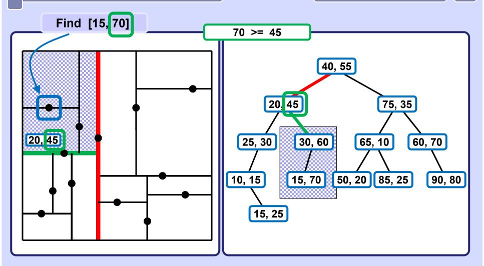
Q = [15, 70], N = [20, 45], Q != N, h(N) = 1. Compare **y-coordinate** of searched key Q to **y-coordinate** of the current node N and continue search accordingly in the left or in the right subtree of N.
