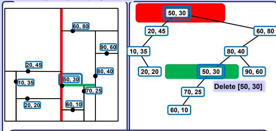
Deleting node [50, 30], it cutting dimension is y, it has no R subtree. Find node Z with minimum y-coordinate in LEFT subtree of [50, 30], Fill [50, 30] with keys of Z and move L subtree of [50, 30] to its R subtree.
