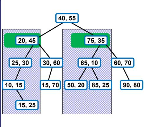
Node with minimal y-coordinate can be only in L subtree of a node N corresponding to cutting dimension y, thus only L subtree of N (including N) must be searched.
