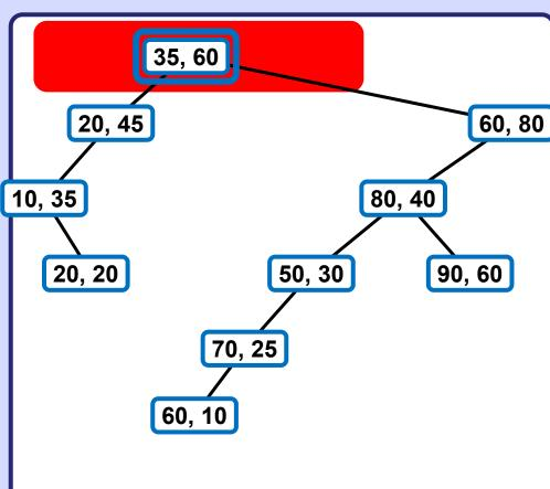
Deleting node [35, 60], its cutting dimension is x.
