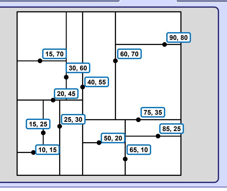
K-d tree is a binary search tree representing a rectangular area in D-dimensional space. The area is divided (and recursively subdivided) into **rectangular cells**. Denote dimensions naturally by their index 0, 1, 2, ... D–1. Denote by R the root of a tree or a subtree.
