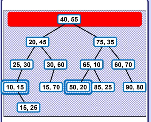
Node with minimal y-coordinate can be in L or R subtree of a node N corresponding to cutting dimension other than y, thus both subtrees of N (including N) must be searched.
