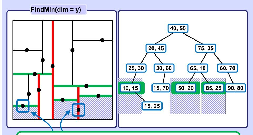
Node with minimal y-coordinate can be only in L subtree of a node N corresponding to cutting dimension y, thus only L subtree of N (including N) must be searched.
