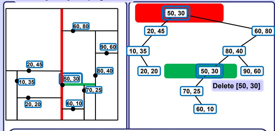
Deleting original node [50, 30], it cutting dimension is y, it has no R subtree. Find node Z with minimum y-coordinate in LEFT subtree of [50, 30], Fill [50, 30] with keys of Z and move L subtree of [50, 30] to its R subtree.
