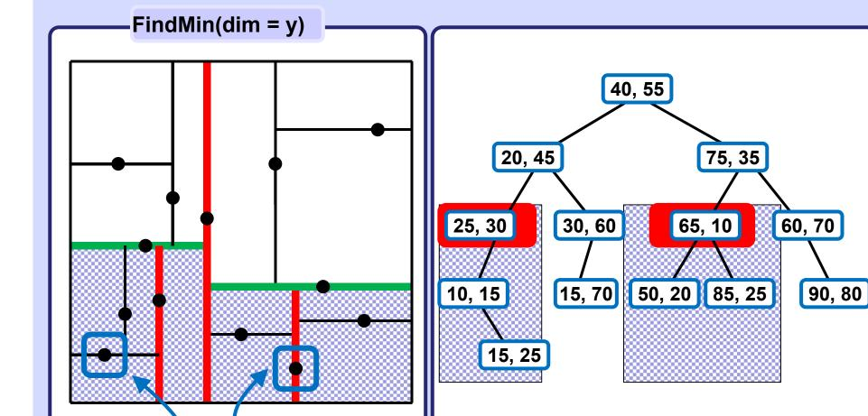
Node with minimal y-coordinate can be in L or R subtree of a node N corresponding to cutting dimension other than y, thus both subtrees of N (including N) must be searched.
