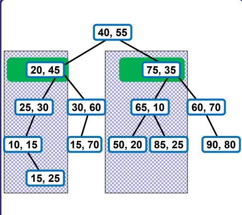
Node with minimal y-coordinate can be only in L subtree of a node N corresponding to cutting dimension y, thus only L subtree of N (including N) must be searched.
