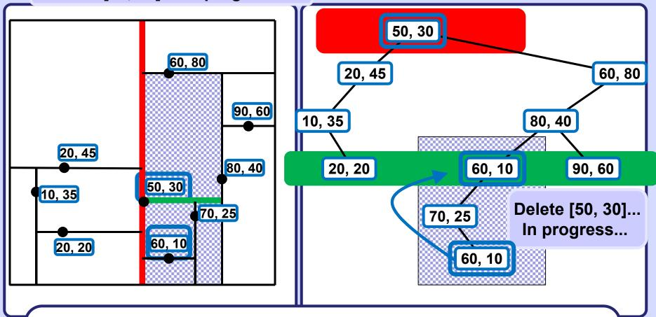
Deleting original node [50, 30], it cutting dimension is y, it has no R subtree. Find node Z with minimum y-coordinate in LEFT subtree of [50, 30], Fill [50, 30] with keys of Z and move L subtree of [50, 30] to its R subtree. If Z is not a leaf continue by recursively deleting Z.
