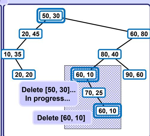
Deleting original node [60, 10], it it is a leaf, delete it and and stop. Note the change in the cell division left to [80, 40], the node with minimal y-coordinate becomes the splitting node for the corresponding area.
