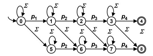
Alternatively: NFA accepting any word containing a subsequence Q which Hamming distance from  $p_1p_2p_3p_4$  is at most 1.
