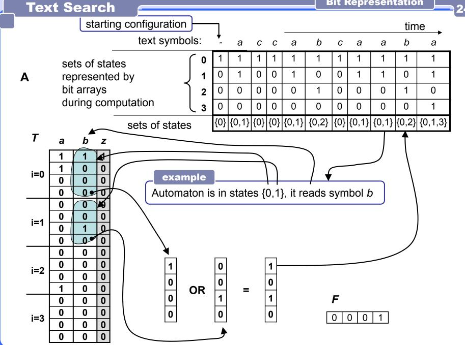
Simulation of work of NFA without  $\varepsilon$ -transitions Basic method, implemented with bit vectors.
