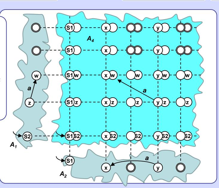
Automaton  $A_4$  accepting binary integers divisible by 3 ( $C_4$ ) in which each symbol 1 is followed by exactly two or three symbols 0 ( $C_2$ ).
