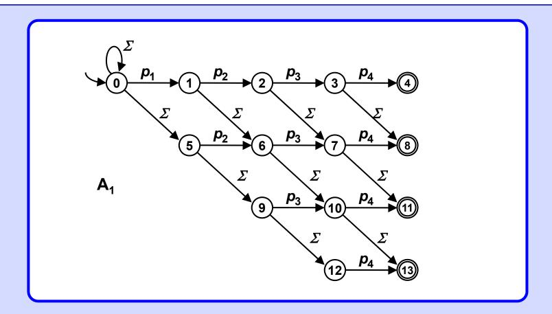
Automaton  $A_2$  for aproximate pattern matching. It detects all occurences of substrings which Hamming distance form the pattern 'rose' is less or equal to 3.
