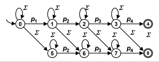
Alternatively: NFA accepting any word containing a subsequence Q which Hamming distance from  $p_1p_2p_3p_4$  is at most 1.
