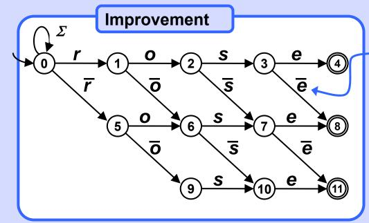
Notation:  $\overline{\mathbf{x}} = \Sigma - \{\mathbf{x}\}$ means: Complement of x in  $\Sigma$ .
