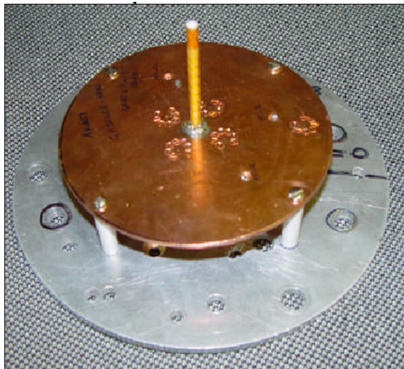
© Jason D. Lohn, Gregory S. Hornby, Derek S. Linden: Human-Competitive Results: Evolved Antennas for Deployment on NASA's ST5 Mission
