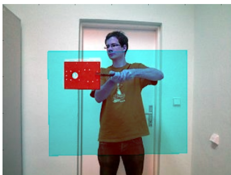
Figure 2: An example of the calibration result. Pixels corresponding to the thermo-camera field-of-view are colored according to their temperature (blue is cold, red is hot).
