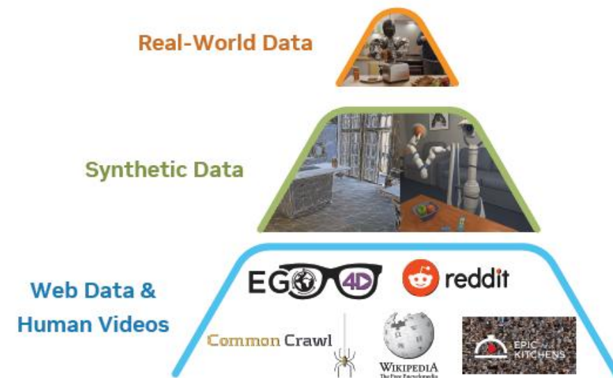
Figure 1: Data Pyramid for Robot Foundation Model Training. GR00T N1’s heterogeneous training corpora can be represented as a pyramid: data quantity decreases, and embodiment-specificity increases, moving from the bottom to the top.
