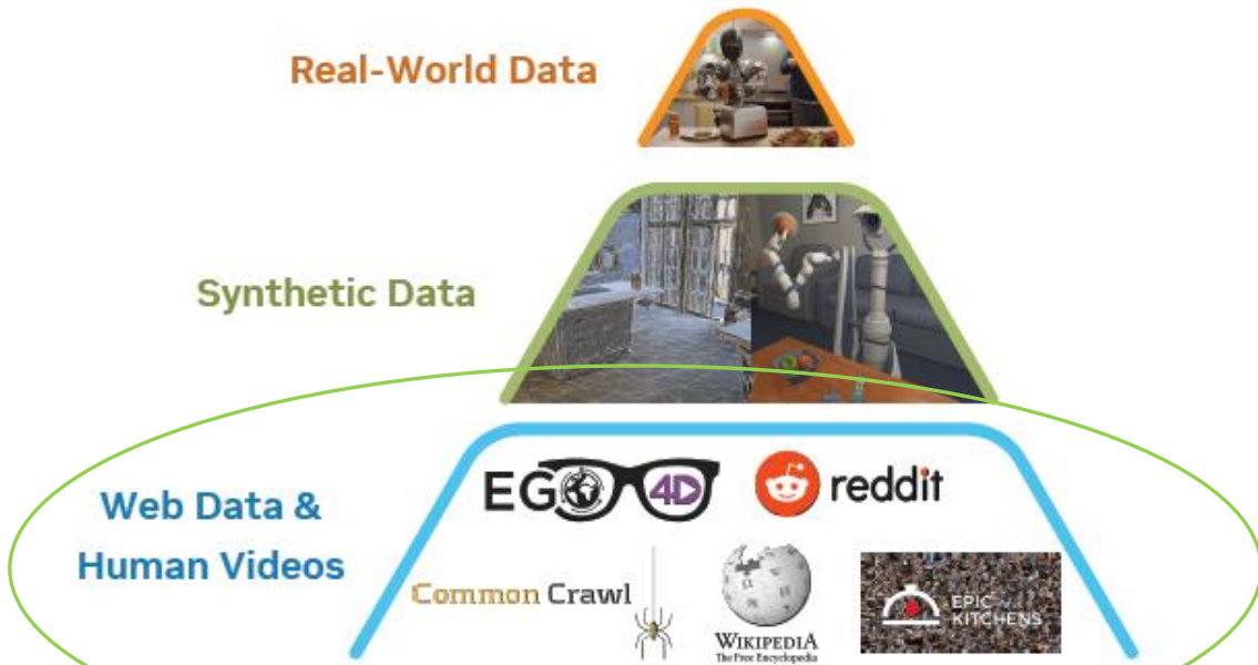
Figure 1: Data Pyramid for Robot Foundation Model Training. GR00T N1’s heterogeneous training corpora can be represented as a pyramid: data quantity decreases, and embodiment-specificity increases, moving from the bottom to the top.
