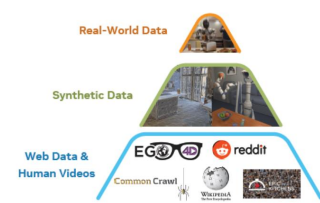
Figure 1: Data Pyramid for Robot Foundation Model Training. GROOT N1's heterogeneous training corpora can be represented as a pyramid: data quantity decreases, and embodiment-specificity increases, moving from the bottom to the top.
