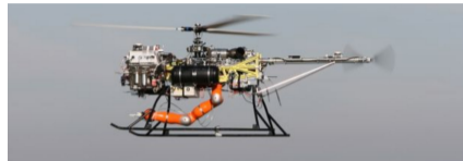
Figure 3: 7-DOF robotic arm under a UAV [3].
