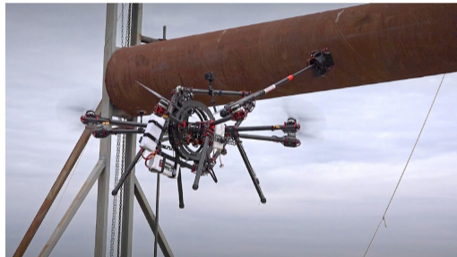
Figure 5: Fully-actuated multirotor UAV applying force to a pipe.
