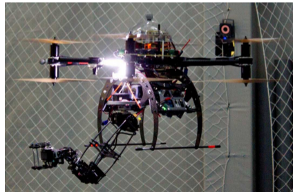
Figure 4: Servo robot arm onboard UAV [4].
