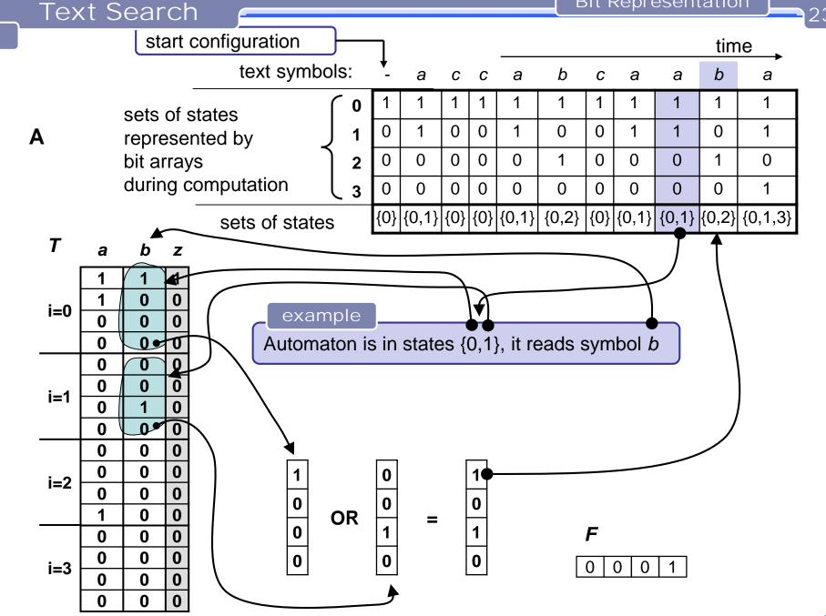
Simulation of work of a NFA without  $\varepsilon$ -transitions Basic method, implemented with bit vectors.
