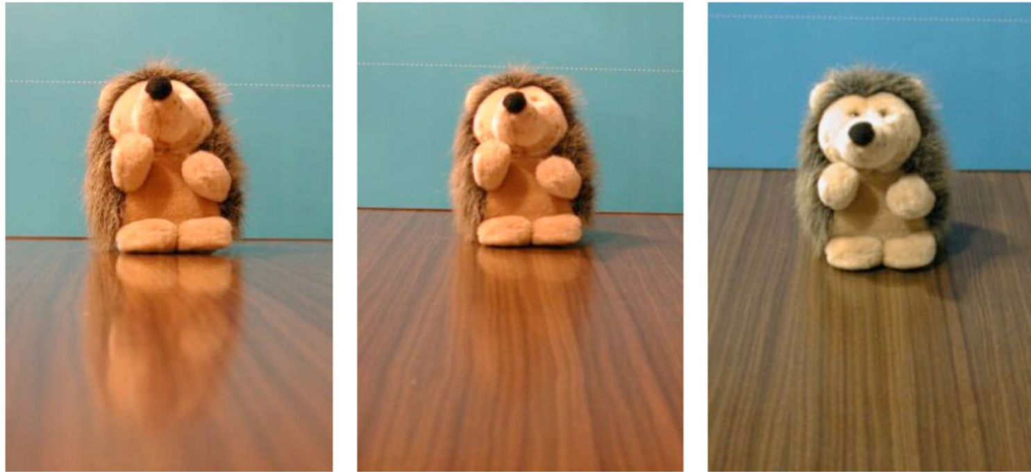
Figure 1: Photos of a specular table from different angles. Note that the table becomes more mirror-like for greater viewing angles
