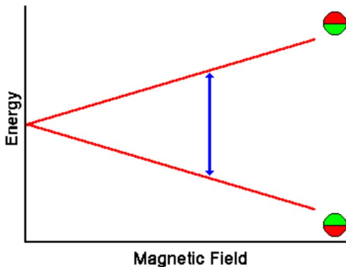
$$f = \gamma B, \quad E_p = hf, \quad \Delta E \propto \gamma B$$
