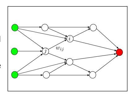
The network defines a mapping  $x_I \mapsto x_T$ , where  $I \subset V$  are the input nodes and  $T \subset V$  are the output nodes of the graph. It is defined recursively by
