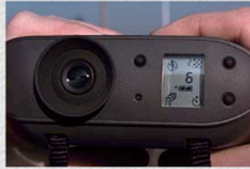
The rear LCD Panel and eyepiece, as seen before putting the camera to the eye.
