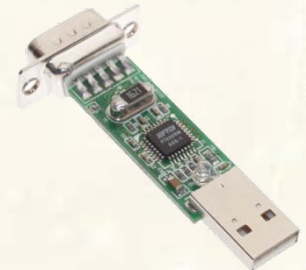
Replacement of missing RS232 port by USB/RS232 converter based on FT232XX chip
