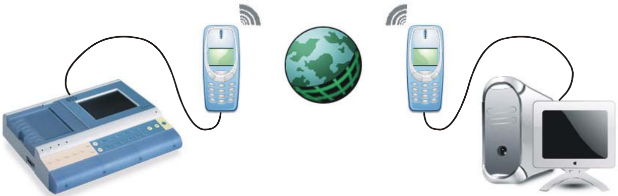
Schematic connection of ECG at the data export to a PC via mobile phone
