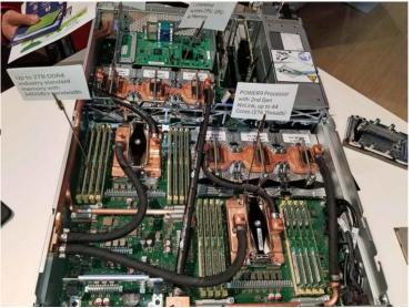
POWER9-SO, Global Foundrie 14nm FinFET, 8×10<sup>9</sup> tran., 17-layer, 24 cores, 96 threads (SMT4) 120MB L3 eDRAM (2 CPU 10MB), 256GB/s
