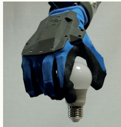
Qb SoftHand (1 motor with position and current sensor)
