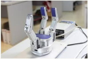
Barrett Hand (96 tactile + 3 fingertip joint torque + 8 joint pos. sensors )
