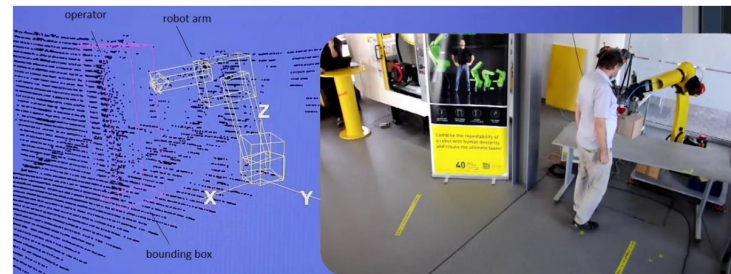
Figure 2: Testing scenario with slow movement of an operator towards a robot arm.
