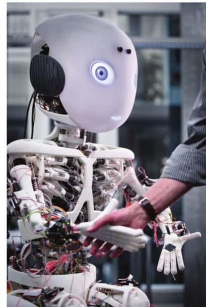
Figure 7. Robo, a human-like, musculoskeletal robot with 28 degrees of freedom and 48 motors, to be controlled by brain-inspired systems. (Photograph courtesy of Adrian Baer.)
