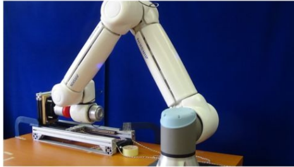
(a) UR10e with AIRSKIN (transient contact).
