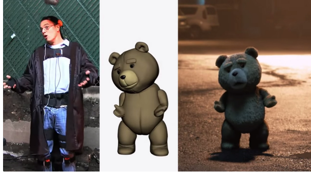
(b) Actor Seth MacFarlane wearing 17 IMUs to capture his motion and animate the teddy bear Ted. The IMUs are placed on different body segments and provide information about the relative position and orientation of each of these segments.
