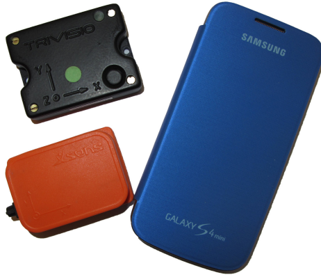
(a) Left bottom: an Xsens MTx IMU [156]. Left top: a Trivisio Colibri Wireless IMU [148]. Right: a Samsung Galaxy S4 mini smartphone.
