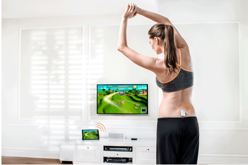
(a) Back pain therapy using serious gaming. IMUs are placed on the chest-bone and on the pelvis to estimate the movement of the upper body and pelvis. This movement is used to control a robot in the game and promotes movements to reduce back pain.
