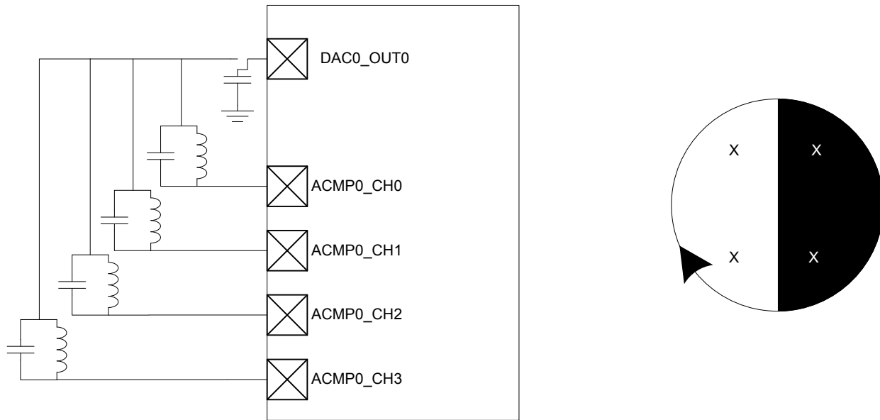
Figure 28.16. LC Sensor Setup
