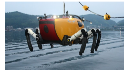
Crabster Underwater inspection
