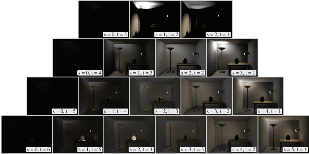
Figure 16.18: Variance Reduction Due to Multiple Importance Sampling. The same sampling strategies as in Figure 16.17, but now weighted using multiple importance sampling—effectively “turning off” each strategy where it does not perform well. The final result is computed by summing all of these images.
