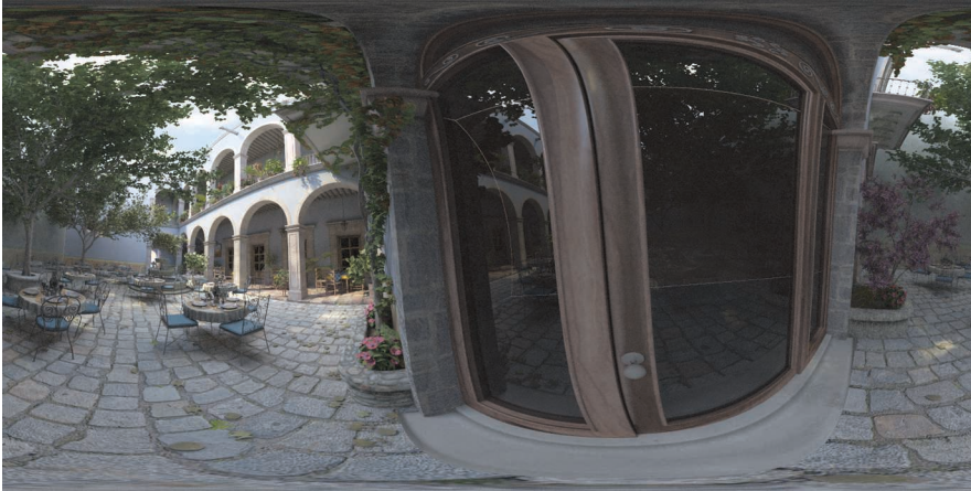
Figure 6.15: The San Miguel model rendered with the EnvironmentCamera , which traces rays in all directions from the camera position. The resulting image gives a representation of all light arriving at that point in the scene and can be used for the image-based lighting techniques described in Chapters 12 and 14.
