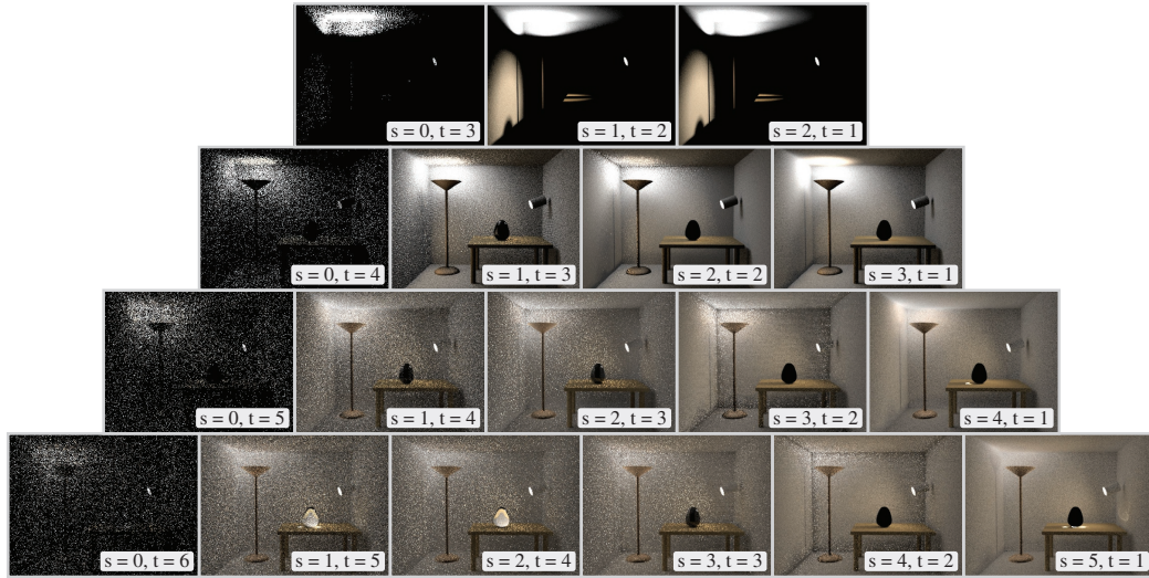
Figure 16.17: The Individual BDPT Strategies. Each row corresponds to light paths of a certain length. Note how almost every sampling strategy has deficiencies of some kind, evident in the form of high variance in these images. (Regular path tracing only samples the s = 1 paths.) Applying multiple importance sampling to path contributions is an effective way to reduce this variance.
