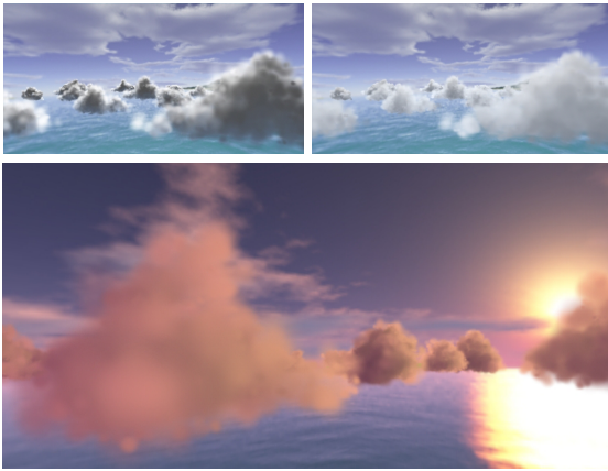
Fig. 12 Shading with only single scattering (left) and with multiple forward scattering (right). Anisotropic scattering simulation with two light sources, orange and pink, to simulate skylight (by Harris and Lastra [30, 31]).
