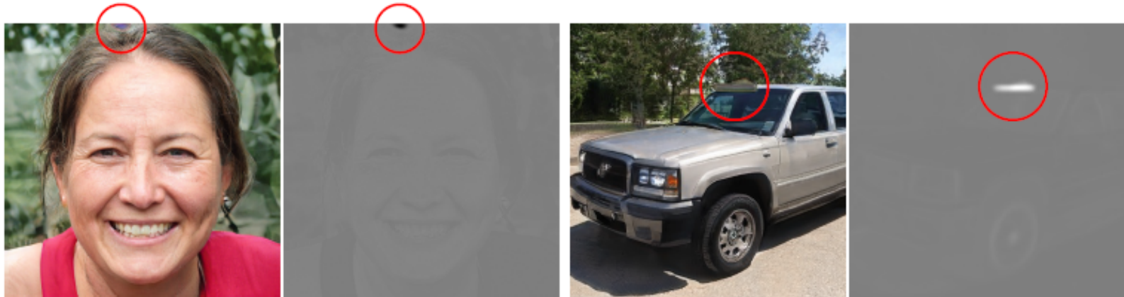
Figure 1. Instance normalization causes water droplet -like artifacts in StyleGAN images.
