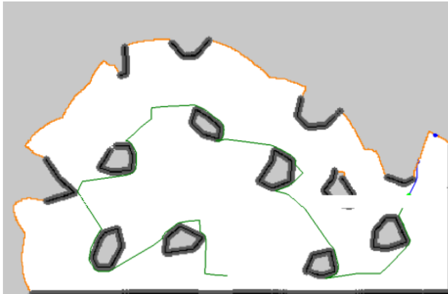
Fig.1.: Terms used in exploration: the white color represents grid cells known to be free, occupied cells are in black and unknown in light gray. Frontiers are in in brown, while the blue dots stand for goal candidates, and the green circle stands for the current robot position. Finally, the already traversed path is in green, while the plan to the chosen candidate is in blue.
